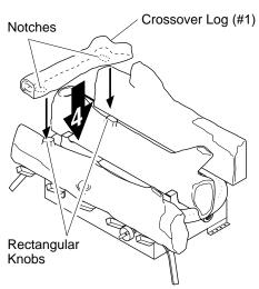
Figure 20 - Installing Crossover Log (#4)
